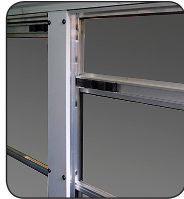
Each window has five open positions. When in any of the top four positions, the window sash can be closed (raised) without retracting the latches.
