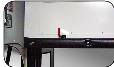
Rotate the lever downward to engage the door mechanism for normal control of the door by the switch panel.
