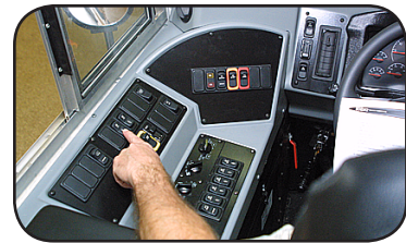
✓ If Vandal lock or other alerts are indicated, turn on dome lights and correct the condition.
