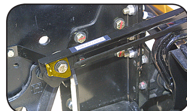
The hold-open strut automatically trips to prevent accidental closure.
