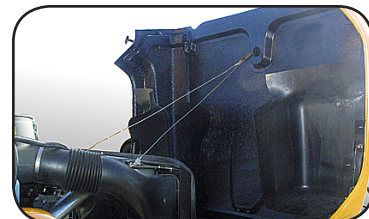
A spring-loaded cable limits the opening range and helps support the hood in the open position.
